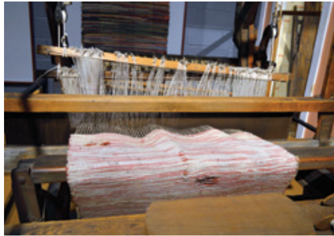
Two-harness loom built by Lithuanian immigrant John Martinkas of West Scranton. All-wooden looms were common in Eastern Europe and many of the Anthracite Region's immigrants brought this tradition with them. The loom was donated to the Museum by the Drazdauskas Family.
